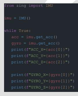
*Example 1.0.15* : reading the 3-axis acceleration.
