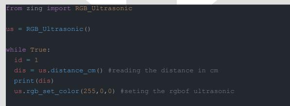
*Example 1.0.16* : Setting up a RGB ULTRASONIC sensor.
