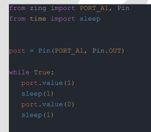
**Example 1.0.1 :** Controlling the GPIO of A1 port. This example shows How to create an LED blinking program using the A1 port.
