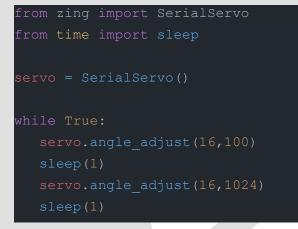
**Example 1.0.16** : Controlling the serial servo motor of zing The above example shows how to set angle to zing.
